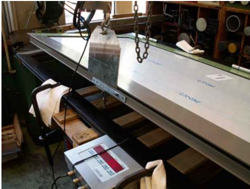
Fig.4.1 Door fixed to steel table
